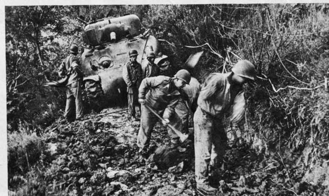
Breaking through to the Gustav Line, tankmen halt to widen a narrow lane. Cast turret of their M-4 looks broad and low, round and flat-topped. A newer turret has two hatches. Standard gun is 75-mm.
